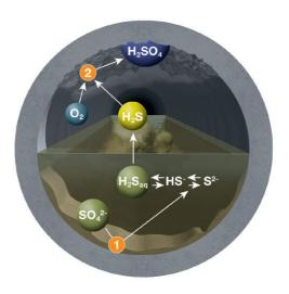
The illustration above represents the different reactions involved in the process of biogenic sulfuric acid corrosion.
